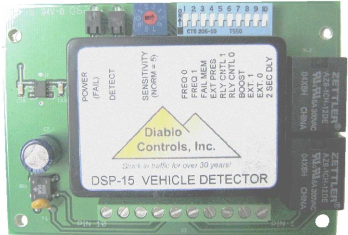
**Sensitivity** - Experience has shown that almost all parking and access control applications can be handled with sensitivity set at NORMAL (level 5). The rotary sensitivity switch is rarely moved from NORMAL. However, the DSP-15 has ten sensitivity settings varying from LOW (level 0) to HIGH (level 9).
